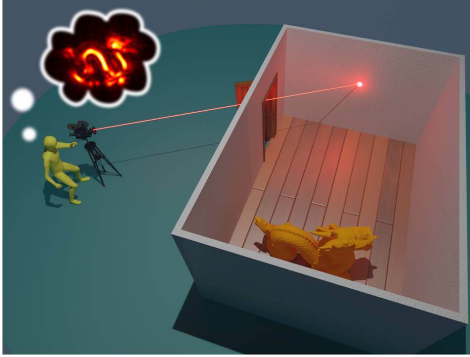
Figure 1.2: Example of a common setup in NLOS imaging. Using a transient camera (dark camera) and controlled illumination (a red laser), the hidden scene (the dragon) can be imaged.
