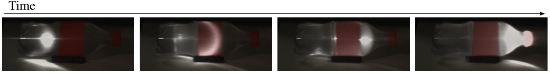
Figure 2.1: A transient imaging capture. A pulse of light enters from the bottom of the bottle (left), and we can see its propagation to the cup of the bottle (right). The effective frame rate of this capture is trillions of frames per second. Results adapted from Velten et al. work [116].
