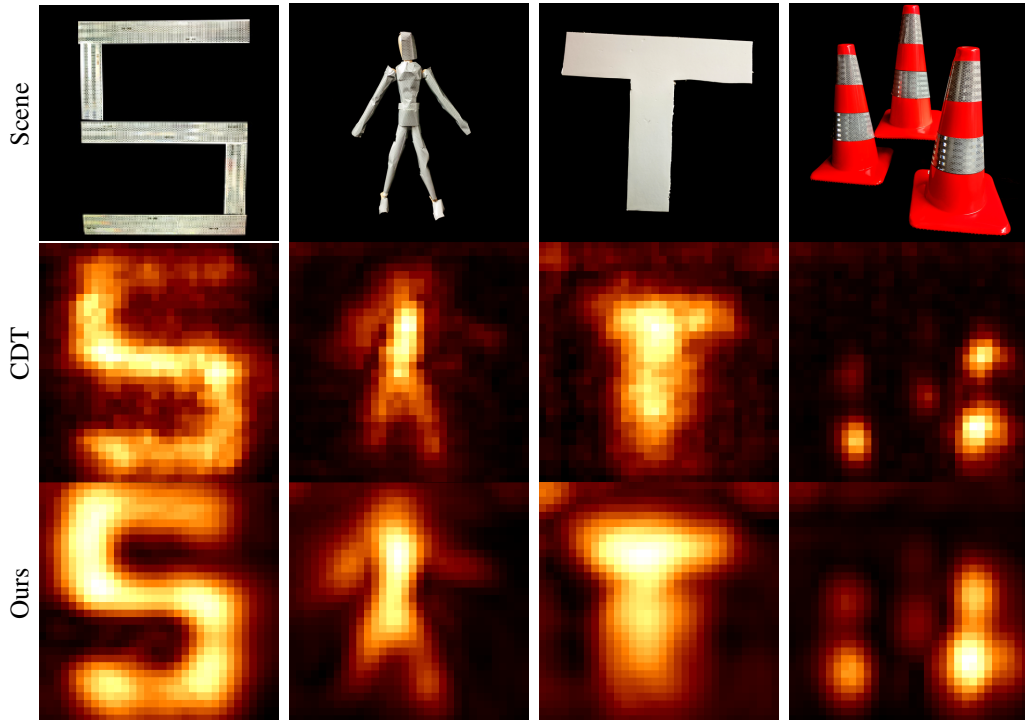
Figure 4.6: Reconstructions of experimental data. Each column is a different scene. Top: images of the scenes behind the diffuser. Middle: Lindell and Wetzstein reconstructions [65] (CDT). Bottom: our reconstructions using Phasor Fields. The higher-frequency of CDT is related to the deconvolution to compensate scattering at the diffuser.
